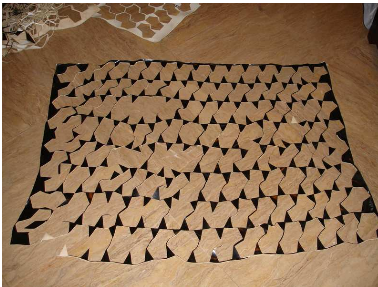
Figure 9: Laminated Sheet Wastage from Cutting Pentagons
