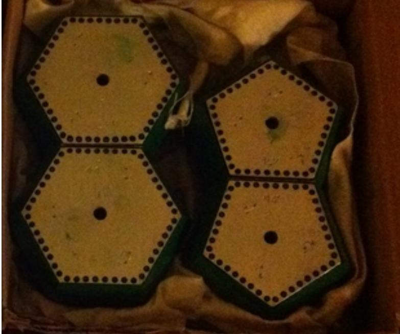
Figure 7: Traditional 2-Hexagon and 2-Pentagon Dies
