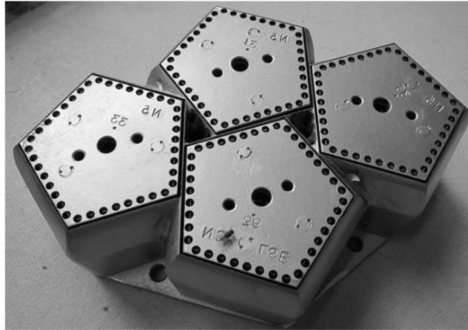
Figure 13: The “Offset” Four-Pentagon Die
