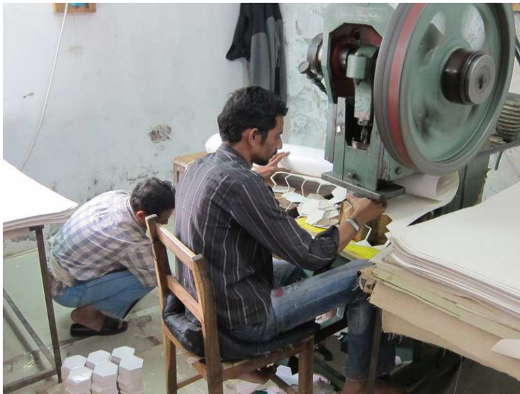
Figure 4: Cutting the Laminated Sheet (Step 2)
